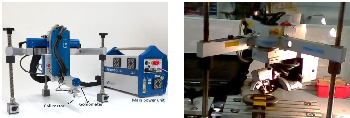
Figure 20 - X-ray diffraction equipment used
