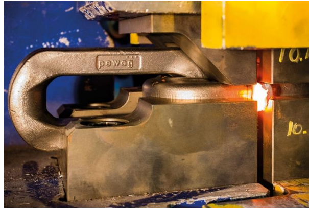
Figure 6 - LFW process applied to "hero" steel chains
